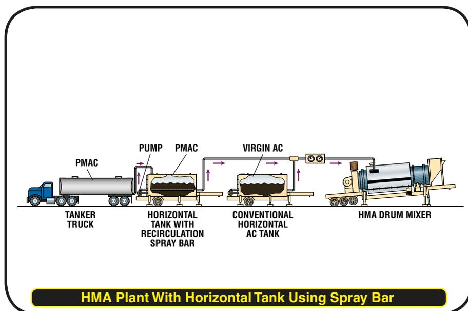
HMA Plant With Horizontal Tank Using Spray Bar
