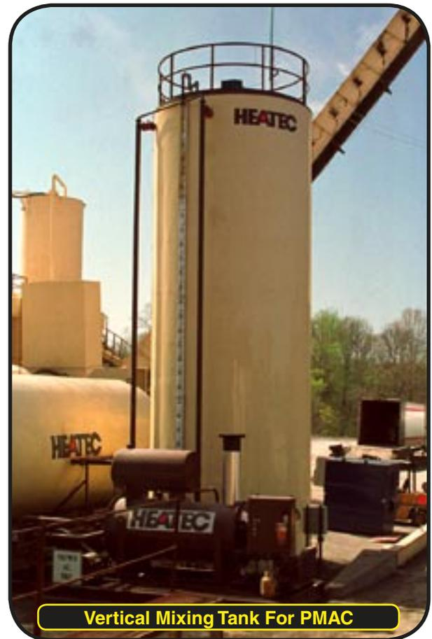
Vertical Mixing Tank For PMAC
