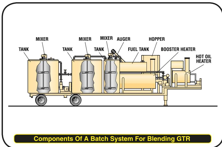
Components Of A Batch System For Blending GTR
