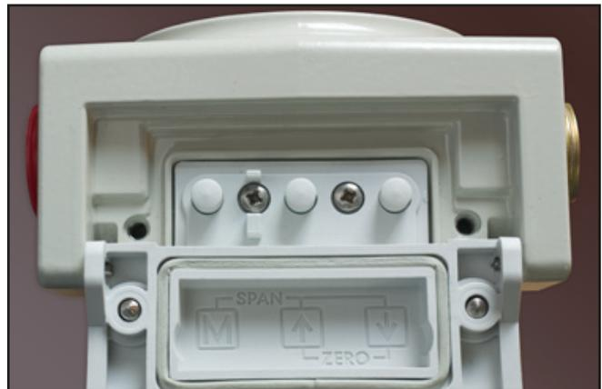
Figure 4. Magnetic pushbuttons.
