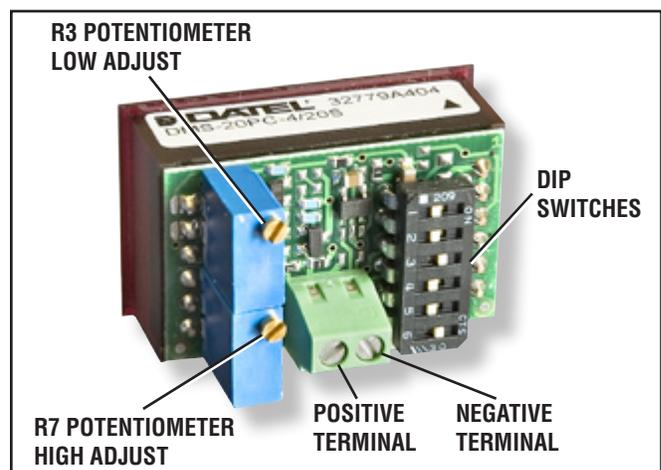
Figure 2. Controls on back of Datel display
