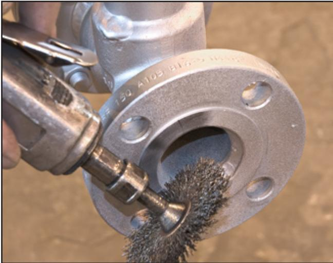
Figure 3. Cleaning surface that mates with gasket.
