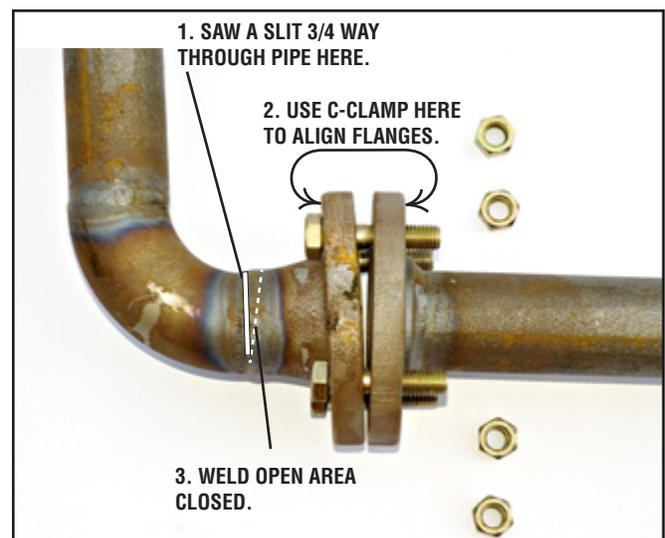
Figure 6. Flanges have unacceptable open angle alignment
