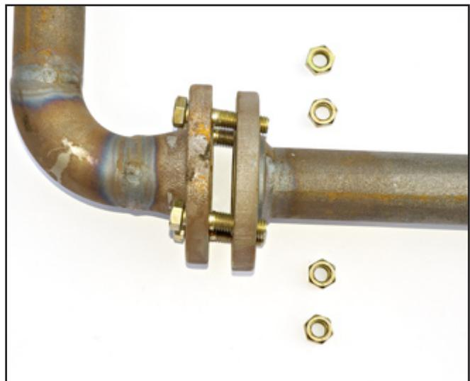
Figure 8. Flanges have unacceptable offset from each other.
