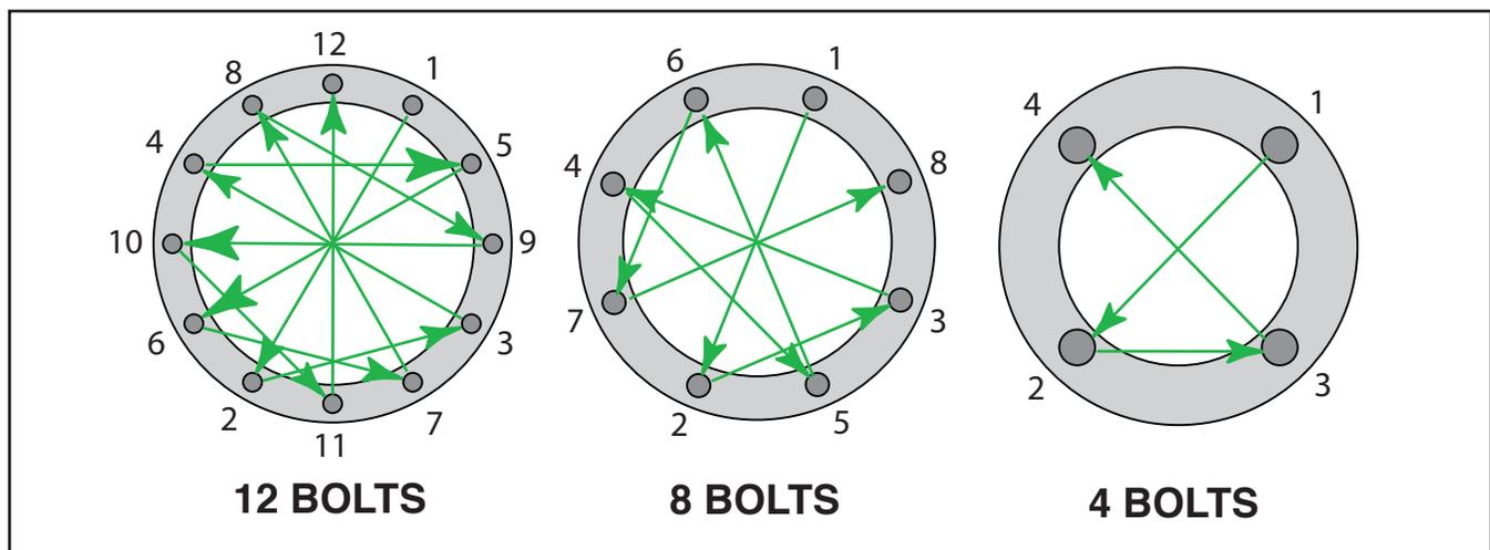
Figure 13. Tightening patterns.
