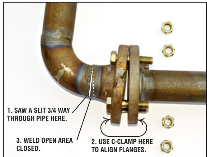
Figure 5. Flanges have unacceptable closed angle alignment.
