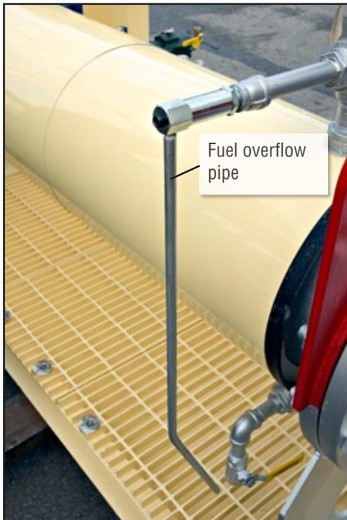
Figure 11. Fuel overflow pipe attached to the pressure relief valve on a skid-mounted preheater.
