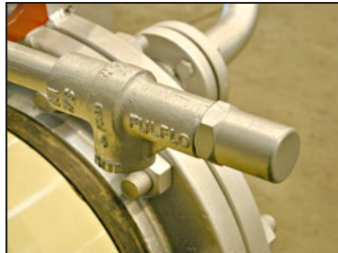
Figure 9. Bypass relief valve used on early model preheaters.
