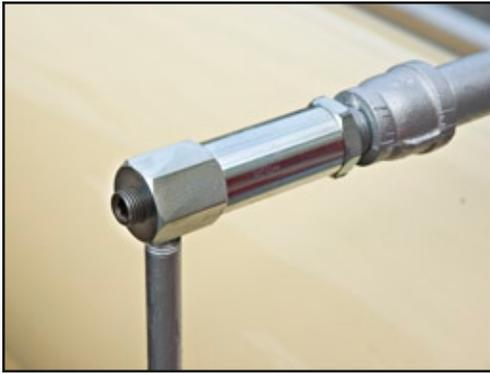
Figure 10. Pressure relief valve used on current preheaters.
