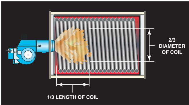
When fired from fuel oil, flame color should be bright yellow. The flame should be centered in the coil.
