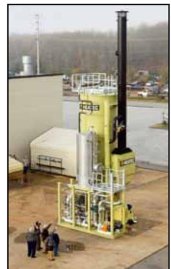
This is a two-pass HMO heater used to remove CO<sub>2</sub> in treatment of natural gas at a facility in California. It is vertically up-fired with an output of 13.4 million Btu/hour.
