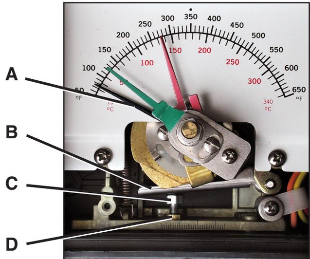
(B) will move the temperature pointer (A). Turn until the pointer indicates the same temperature as the thermometer next to the dry well. **Note:** It is generally best to adjust the temperature pointer from slightly *below* the proper temperature *up* to the proper temperature.
