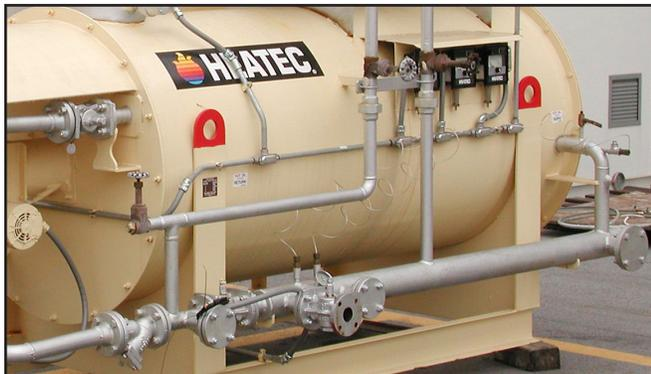
in dry wells in the heater hot oil piping to sense oil temperature. Next to these dry wells are thermometers needed to aid in calibrating the controllers.
