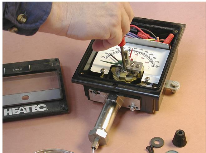
Loosening the screw that secures the pointer.
