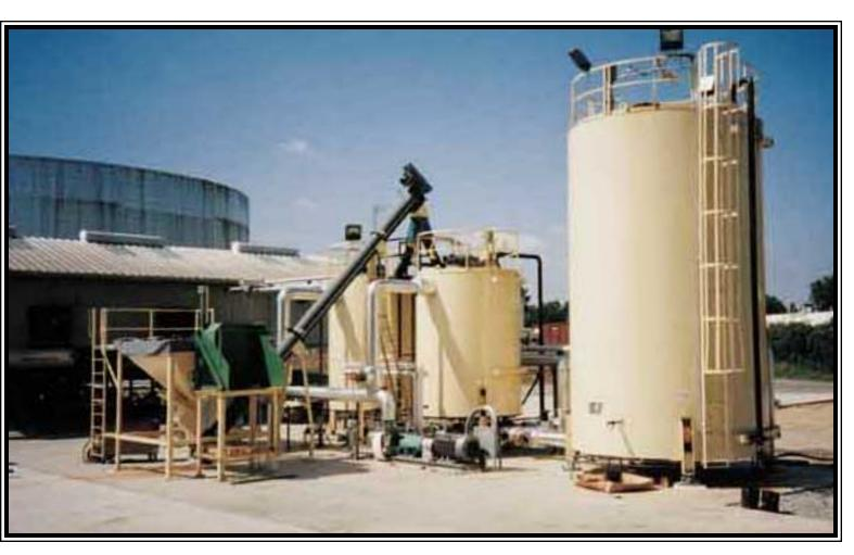
"Generally speaking, we add certain modifiers to the asphalt cement while utilizing elevated temperatures and high-shear mixers to change the molecular structure of both the asphalt and the modifiers. In this way, the modifiers—which are usually a polymer of some sort—and the asphalt cement are brought together so that they become one entity, instead of two.
