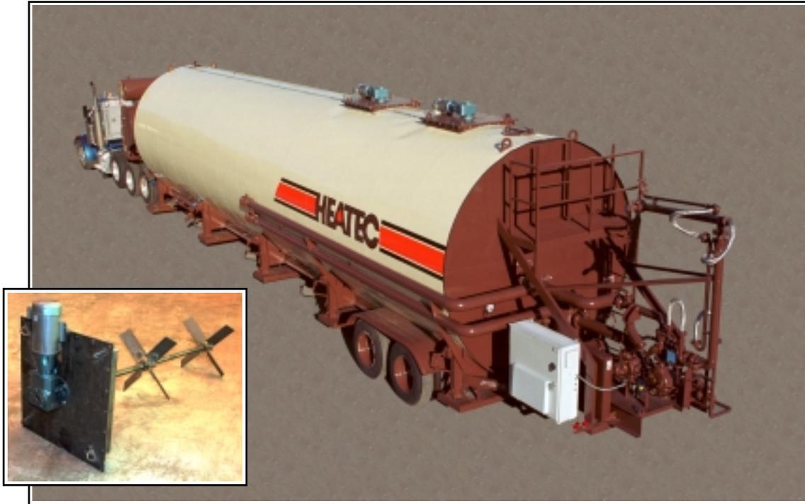
Heatec Heli-Tank™ for portable HMA plants using modified asphalts. It has a forward compartment and a rear compartment, which are independently heated and controlled. The forward one is for virgin asphalt and holds 20,000 gallons. The rear one is for GTR asphalt and holds 15,000 gallons. Two factory-installed mixers are designed and positioned in the rear compartment for optimum mixing efficiency.
