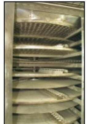
Drying trays used to make polyaspartate polymer
