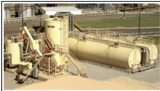
L to R: Heatec polymer blending system with two 4,000-gallon vertical batch tanks, one 22,000-gallon blending tank, and two 35,000-gallon horizontal asphalt tanks. The polymer feed system is in front of the two batch tanks.
