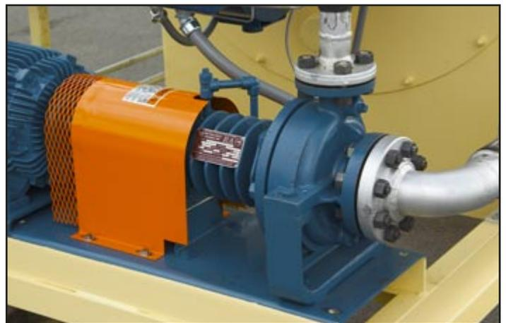
Dean and Sihi centrifugal pumps are standard for our heater. The one shown here is a Dean pump with mechanical seals.
