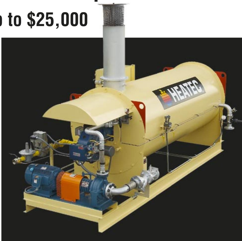
The heater has a helical coil made and tested at our factory. It meets ASME code and has a warranty based on thermal fluid operating temperatures: 1 year for 650 degrees F; 2 years for 550 degrees F; or 3 years for 450 degrees F. The coil is protected by a pressure differential switch shown on the side of the heater. It shuts down the burner in the event of a problem that causes abnormally low flow through the coil.
