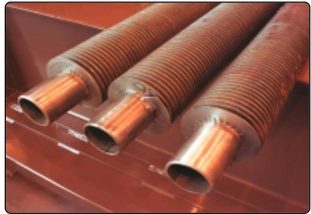
Serrated fins are shown here. The serrations increase efficiency even more than solid fins by increasing the turbulence of liquid flowing around the fins.
