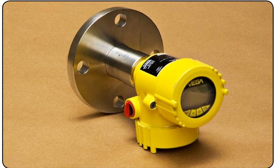
**Radar sensing unit.** Mounts atop the tank and emits a microwave signal, which travels downwards until it reaches the surface of the liquid asphalt. The signal is reflected back to the unit by the surface of the asphalt. The reflected signal is read by the unit, which converts the signal to data related to the distance traveled. This information is converted as needed for the various types of remote displays, including the unit's built-in display.
