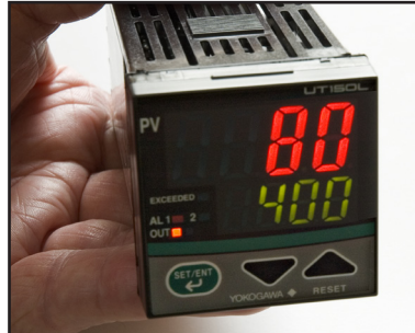
Figure 1. Yokogawa UT150 controller.
