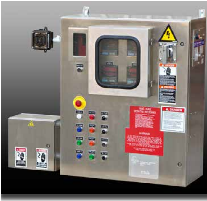
A typical NEMA Type 4 panel for areas temporarily exposed to combustible gases. Panel is equipped for Type Z pressurization and also purges the small panel on the left.
